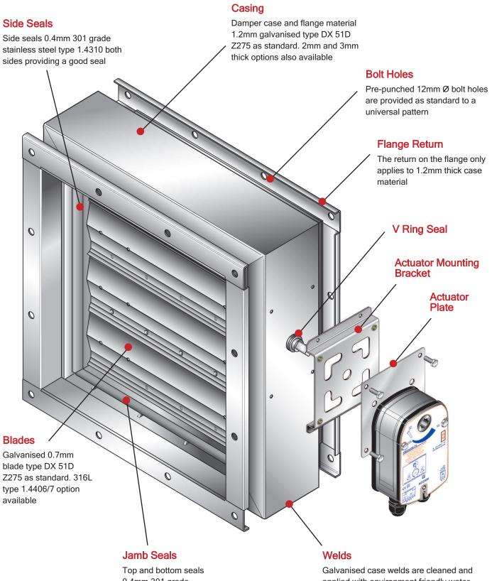
0.4mm 301 grade stainless steel type 1.4310 providing a good seal Galvanised case welds are cleaned and applied with environment friendly water based paint.
