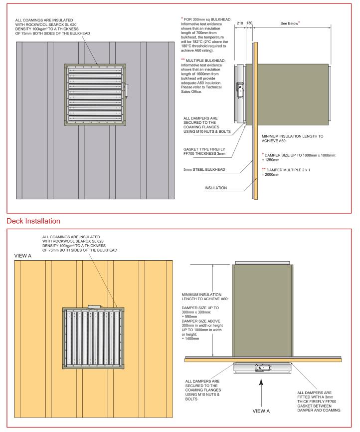
The bulkhead and deck to be in accordance with FTP code 2010 Figure 12. Insulation material and thickness for the bulkhead and deck should be in accordance with the manufacturers instruction. The length specified is required to achieve A60 classification. For AO classification, insulation is not a requirement.
