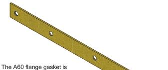
an accessory for mating dampers to bulkheads for an even seating and to provide galvanic isolation, typically required in marine applications. Supplied in plain strips with or without matching holes to suit the BSB damper flange.
