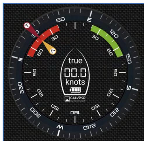
This shows the values of the Real and Apparent wind. The external circle is the compass, showing the north position (in degrees). The internal one is used by the Real and Apparent wind markers (red and yellow respectively) to show the direction of the wind (in degrees).
